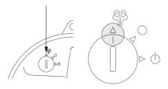
If the control knob is left in the off position  $\bigcirc$  or standby  $\bigcirc$  position the water will not be heated.
