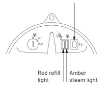
2. Turn pointer on control knob to steam position (3), amber steam light will illuminate.
